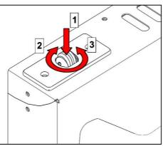
Figure 7 – Door catch adjustment.
