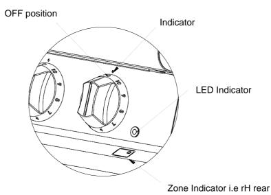
When a cooking zone is switched on, the LED indicator will light and stay lit during heating/cooking. If a pan is removed from the zone, the LED will flash approximately once per second. This will indicate that the cooking zone is still active and is awaiting detection of a pan.
