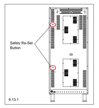
9.13.1 An overheat safety trip is fitted to the oven. Access is at the rear of the appliance as shown. To reset, press button. (See warning note below).
