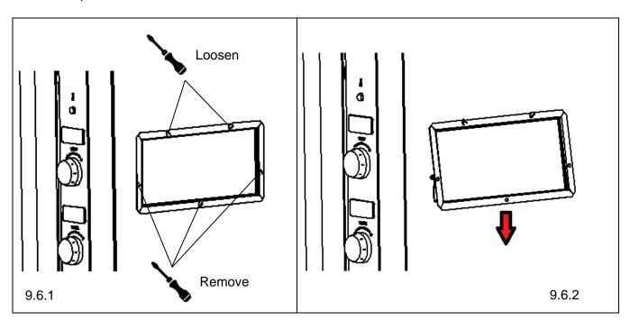
9.6.2 Pull panel out at bottom and slide down.
