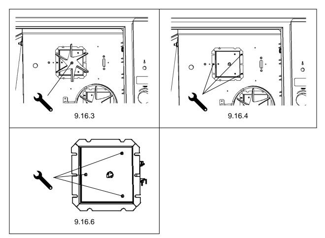
9.16.2 Remove element surrounding fan that is to be replaced.
