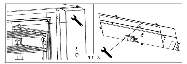
9.11.3 Fix spanner on nut inside chamber and fix spanner on nut outside chamber and turn to remove operating thermostat.
