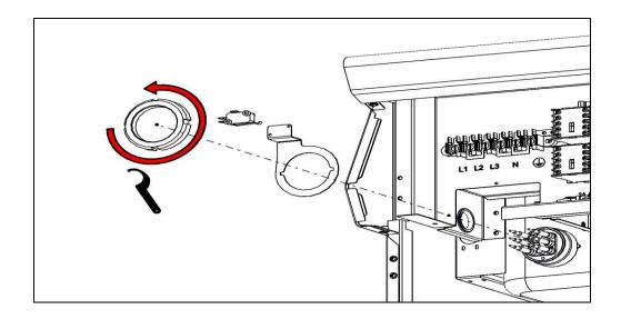
7.7.2 Remove ring nut and safety switch as shown.
