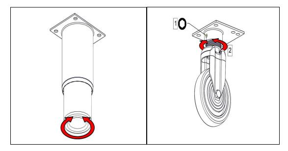
6.2.2 Fit anti tilt device as shown below.
