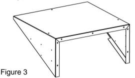
Hold bracket against wall in desired position. Ensure top surface is horizontal in both directions. Use bracket as a template to mark fixing hole positions. Drill and plug wall to accommodate fixture of bracket.
