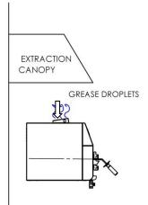
EXTRACTION Diverter prevents droplets falling into burner. GREASE DROPLETS
