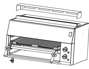
Fit diverter over flue with slots to rear
