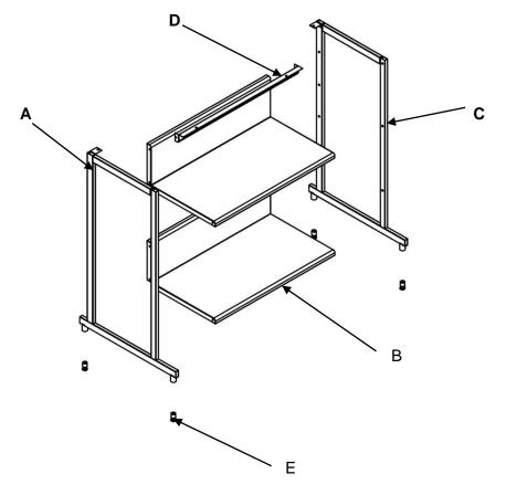
a) Fix both shelves (B) to end supports (A & C) using M5 screws provided.
