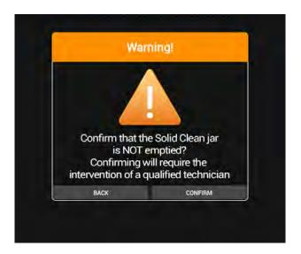
If the Solid Clean jar was not emptied, the detergent creation procedure did not complete correctly. Confirm the choice by pressing "CONFIRM" or press the "BACK" button to change the choice.
