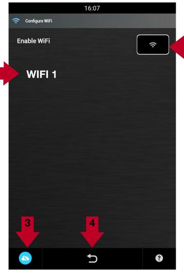
Press the icon (1) setting it to **ON** to activate the Naboo Wi-Fi connection
