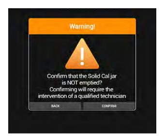
If the Solid Cal jar was not emptied, the descaler creation procedure did not complete correctly. Confirm the choice by pressing "CONFIRM" or press the "BACK" button to change the choice.
