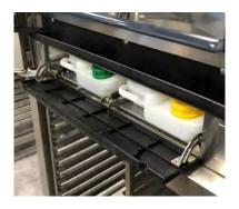
Put the cartridge back in is slot and close the small door and the oven door.
