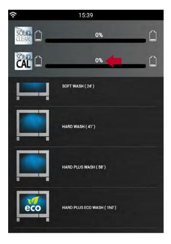
Select **CALOUT** or the **WASH+CALOUT** desired. If there is insufficient descaler to run the wash, a popup appears requiring the Solid Cal descaler generation procedure.
