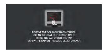
Once the detergent creation process is complete, remove the Solid Clean jar, clean around the drawer cap and thoroughly rinse the cap.
