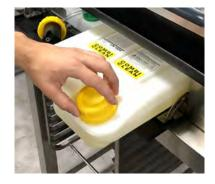
Remove the top of the new cartridge.
