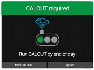
When the **CALOUT** process is needed, a popup warning appears: "Perform CALOUT by the end of the day". Press "Start CALOUT" (see next paragraph) to immediately perform CALOUT or press "Ignore" to perform the procedure later (example: at the end of the day).
