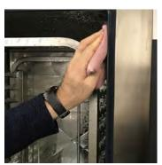
In floor-standing appliances, always fully insert the trolley until it comes into contact with the front gasket and block the wheels. Partial insertion of the trolley may cause damage to both the front and doormounted gasket.
