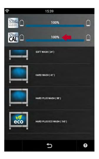
Once descaler creation is properly completed, the level is reset to 100%.
