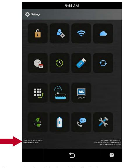
Check the software version shown in the lower left on the display.
