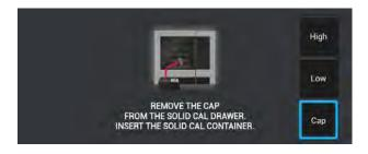
Open the drawer and remove the cap from the SOLID CAL drawer.
