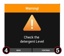
If the cartridge/canister is empty, press "BACK" **(4)** and replace it by following the instructions in the paragraph "REPLACING THE DETERGENT/DESCALER CARTRIDGE" **(5)** before starting the wash cycle.
