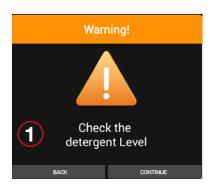
If there is not enough detergent to run the selected wash cycle, a popup window will appear on the display telling you to visually check the detergent/descaler level (1).
