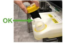
Insert the cap with the extraction system (YELLOW for COMBICLEAN detergent and GREEN for CALFREE descaler) ensuring that the clear extraction pipe is facing the front of the cartridge as shown in the figure.
