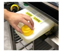
Remove the top of the new cartridge.
