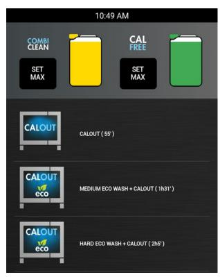
Select **CALOUT** or the desired **wash** + **CALOUT** and the washing procedure starts.
