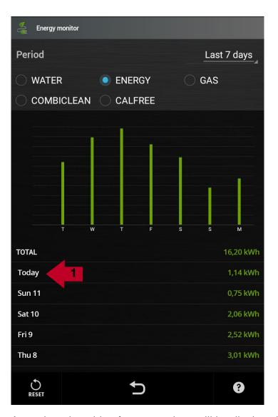
The Energy Monitor allows you to view the information about oven consumption in a specific period.
