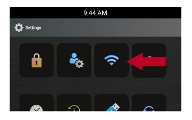
Press the icon "Wi-Fi Settings" to check the activation and availability of the Wi-Fi connection.
