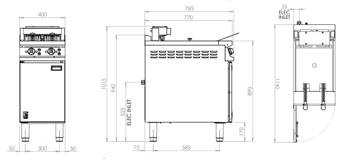
Measurements in mm Unit on castors is the same hob height
