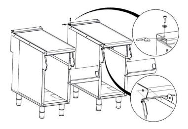
NOTE: The DLS system is designed to give a quick and easy suiting solution. If you require an improved seal between appliances we recommend you use, a food grade, high temperature silicon sealant. This can be supplied by Falcon part no – 523400021
