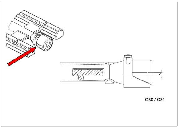
8.1.5 When replacing burner, ensure locating lugs locate in the rear support bar correctly.
