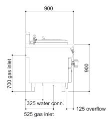
The unit can be connected a the rear or from below
