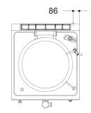
The unit can be connected at the rear or from below
