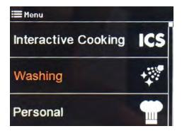
Turn knob **16**, select the wash required displayed on display **15** and confirm the start by pressing knob **16**.
