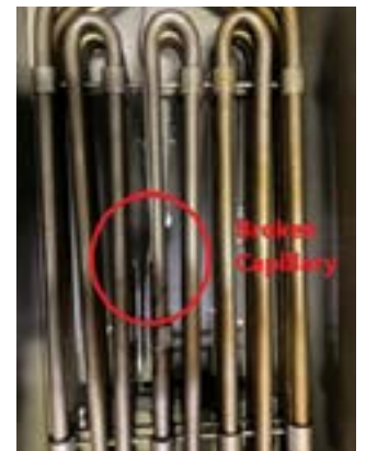
Electric fryer - Safety thermostat, broken capillary.
