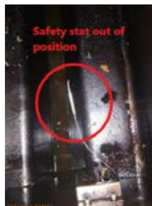
Electric fryer - Safety thermostat, broken capillary.
