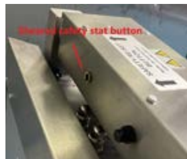
Electric fryer – safety stat reset button sheared off due to stowing fryer lid behind element head
